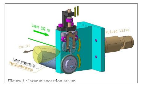
pulsed evaporation setup is used to provide an intense a stable source fragile molecules cooled at ~20K by supersonic expansion. The molecules are examined by laser ionization, time of flight mass spectrometry and
